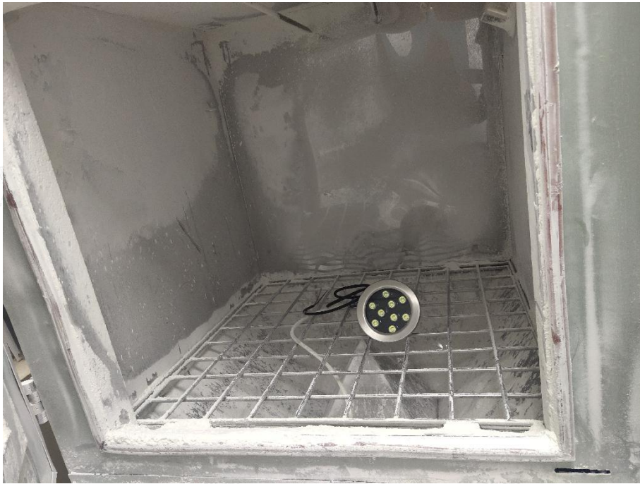
Photo 3: IP6X test of model 61063
