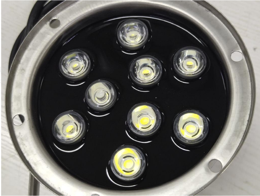
Photo 5: Test result after IP6X and IPX8 test
