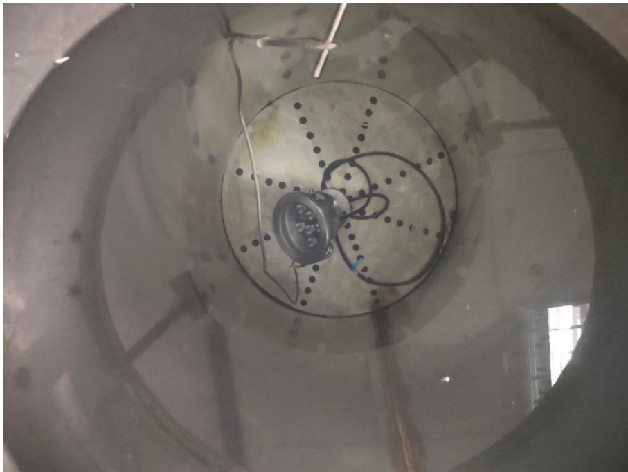
Photo 4: IPX8 test of model 61063
